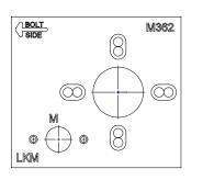
The illustrated template is positioned for a Right Hand mounted lock but can be rotated to drill a lock mounted Left Hand, Vertical down or Vertical up.
